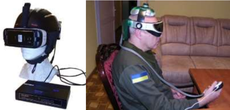
Fig. 7. – General view of the helmet and control unit on the demo stand (left) and testing the prototype helmet (right)
